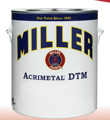
A premium, rust-inhibitive, interior/exterior acrylic coating. Acrimetal is formulated for direct application to bare metal and metal with tight rust. Acrimetal is extremely durable, has excellent adhesion to metal and galvanized surfaces and contains rust inhibitive pigments for added protection. It is a versatile replacement for conventional solvent-borne industrial primer/finish systems.
